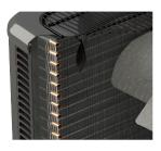
Franklin's 5mm tube condensing coil design optimizes the heat transfer ability of R-410A refrigerant compared to standard 3/8" copper tubing.
