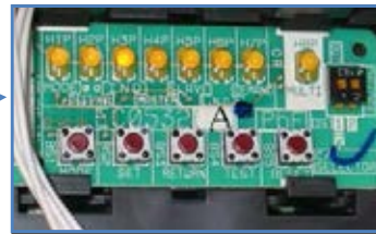
H1P to H8P LEDs MODE-SET-RETURN-TEST & RESET buttons
