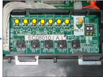
H1P to H8P LEDs MODE-SET-RETURN-TEST & RESET buttons
