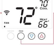
Fan on — Low speed Pressing the fan button again will cycle through fan speeds.
