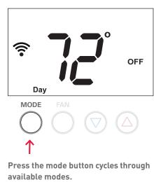
As each mode is selected, its name appears in the upper left corner of the display. The text disappears 1 second after the mode is selected, but the relevant setpoints for the selected mode are always displayed.
