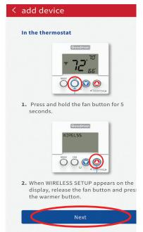
2. Press and hold the fan button on the thermostat for 5 seconds to put the thermostat in "Wireless Setup" mode. Then press the up/ warmer button on the thermostat to display the 6-digit pairing code and select "Next".
