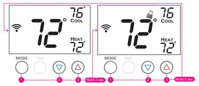
**To disable, or "lock" the keypad,** press the warmer (up) and cooler (down") buttons and hold for two seconds. When the lock icon appears on the display, release the buttons.
