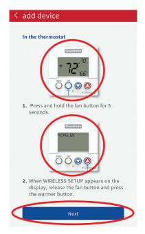
**4. Press the fan button** for 5 seconds to put the thermostat in "WIRELSS SETUP", then select "Continue".
