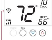
Fan on — High speed Pressing the fan button again will cycle through fan speeds.
