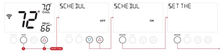
Press and hold the fan and warmer (up) buttons for 2 seconds to enter schedule mode for programming a schedule. While in schedule mode, press the mode button to advance through each setting for each day of the week and each time period of each day.
